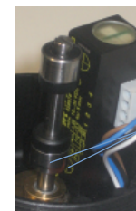
Target switch and cam for open valve
