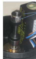
Target switch and cam for open valve
