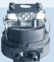
Control head without cover, 5-pole DeviceNet connector, PG9 for cable bushing from outside
