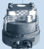
Control head without cover, ASI special connection 2, M12 flanged connector, 4-pole, PG9 for sensor cable bushing from outside
