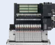
Type 8640 AirLINE Quick with 12x 2x3/2-way valves with Profibus DP and 24 digital inputs
