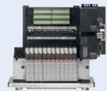
Type 8640 AirLINE Quick with 12x 2x3/2-way valves with Profibus DP and 24 digital inputs
